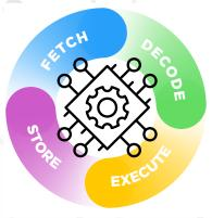
At the core of all microcontroller architectures is the fetch, decode, execute and store cycle. In this cycle, the processor fetches an instruction from RAM and stores it in registers.
